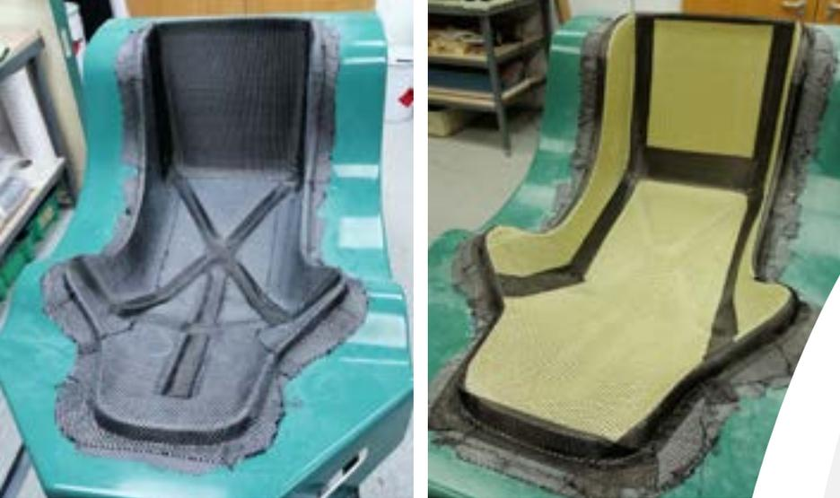
Car Seat mould tooling by J-TEC Composites
