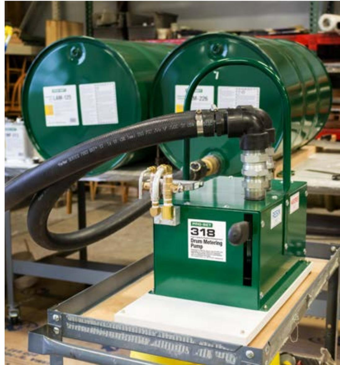
*318 Drum Metering Pump and example setup. Chemical resistant hoses and plumbing fittings are not included as each setup will need to be customised for the fabricator's needs.*
