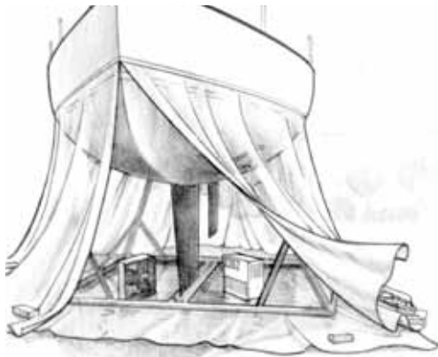
Figure 5.1. Drying the hull can be accelerated by tenting the hull with a plastic skirt taped just above the waterline.
