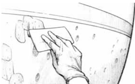
Figure 6.2 Use a squeegee to apply fairing compound, and slightly overfill the area. Shape the mix to blend with the surrounding contour.
