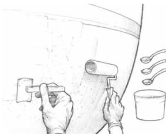
Figure 7.4. Add 422 Barrier Coat Additive to the second and remaining coats to increase moisture exclusion effectiveness and abrasion resistance.
