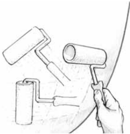
Figure 6.1 Wet out the surface with resin/hardener mix. to avoid sags, allow the wet-out coat to gel before applying fairing compound.
